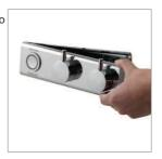
To remove the controller from the back plate, undo the screw and remove from the base of the controller assembly. Carefully pull the controller away from the back plate and set aside.
