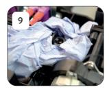
Place cloth around the thermistor housing and ensure the power pack is protected.
