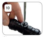
Observing the thermistor housing just partially open the cold water isolation valve
