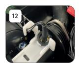
Check the o-ring seal is still seated in the thermistor housing. Plug the thermistor back in and re-fit the thermistor clip, ensuring the clip locks into position.
