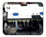
Ensure that all wiring connectors to the Logic Module have not come loose and are pushed home.
