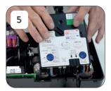
Remove the logic screw and fold the logic out of the way.
